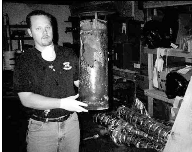
Bruce Andrews holds a trophy duct; fixing holes this big can cause unintended problems.
