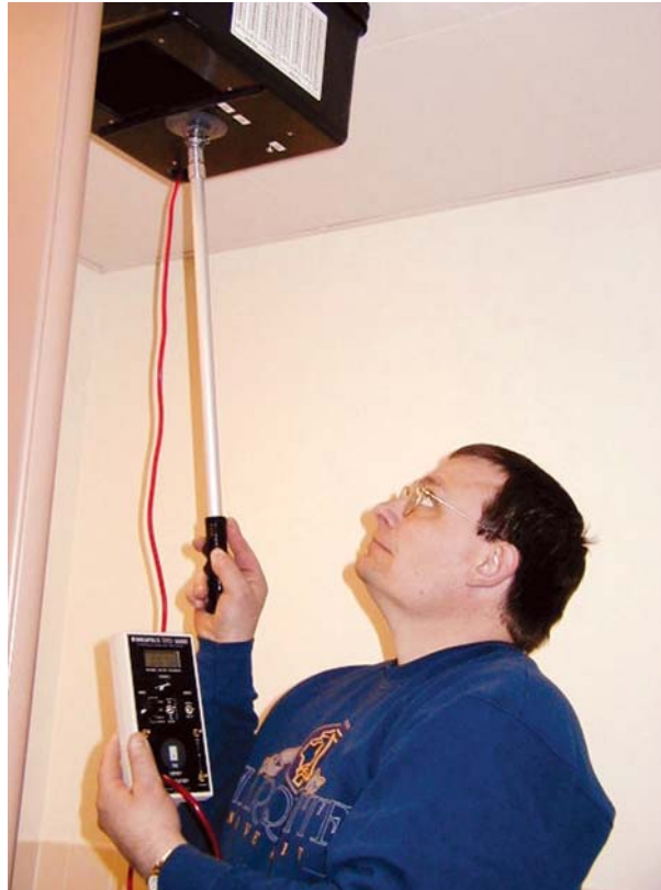
Robert Parkhurst measures exhaust ventilation. In July 2005, Wisconsin's Home Energy Plus Weatherization program began to move away from a building tightness guideline to a ventilation standard in evaluating its weatherization efforts.
